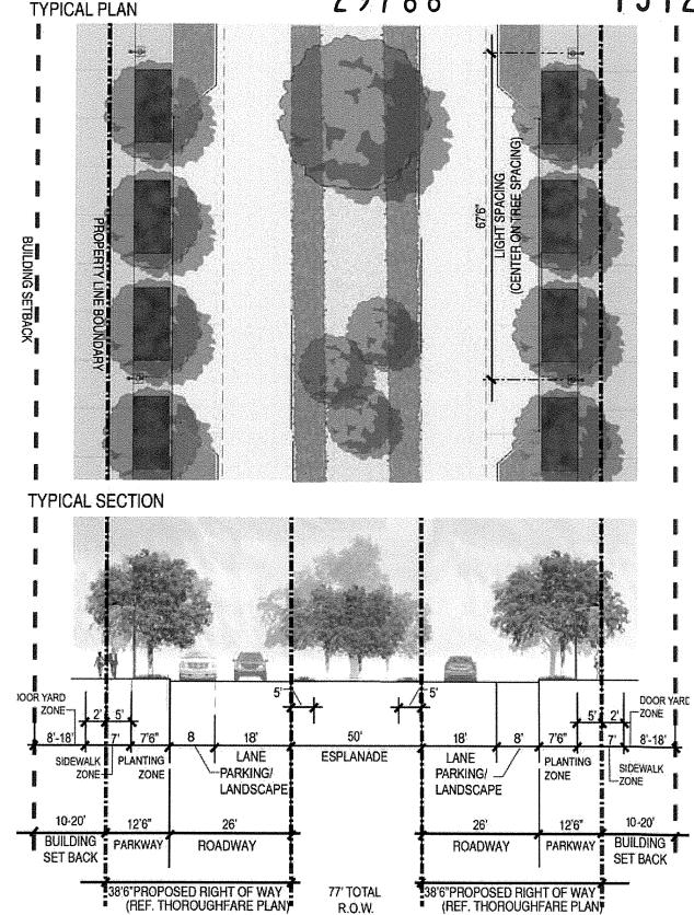
ON-STREET PARKING ZONE CAN BE REPLACED WITH AN ENLARGED LANDSCAPE ZONE. U-TURN LANE REQUIRED AT INTERSECTION OF FN5.
