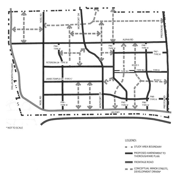
\* THESE MINOR STREETS ARE CONCEPTUAL AND INTENDED ONLY TO ILLUSTRATE DESIRED CONNECTIVITY FOR NEW STREETS. ALTERNATIVE ALIGNMENTS MAY BE APPROVED BY THE DIRECTOR OF PUBLIC WORKS IF THEY PROVIDE EQUIVALENT CONNECTIVITY AND COMPLY WITH THE PROVISIONS OF SECTION 51P-887.115 (STREET STANDARDS) AND SECTION 51A-13.502 (NEW MINOR STREETS).
